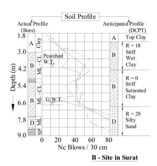
Fig. 4: Sol Profiles Developed by DCPT
