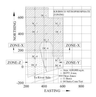
Fig. 2: Typical Zoning Plan by DCPT to Plan Detail Exploration (Desai M.D.)
