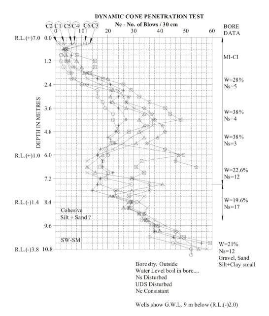
Fig. 6 Chart showing DCPT tests result for foundation of high-rise building at Surat.
