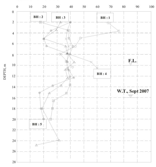
Fig. 5: Standard Penetration Test Data for the Building at Dwarka, Delhi.
